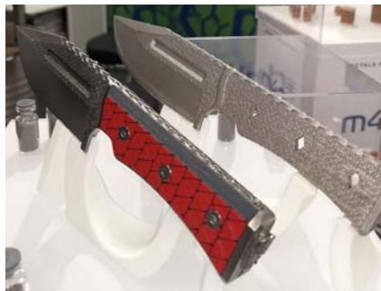
Img.: additive manufactured knife,
