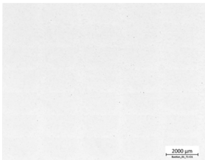
Image: Microsection; porosity < 0.04%
